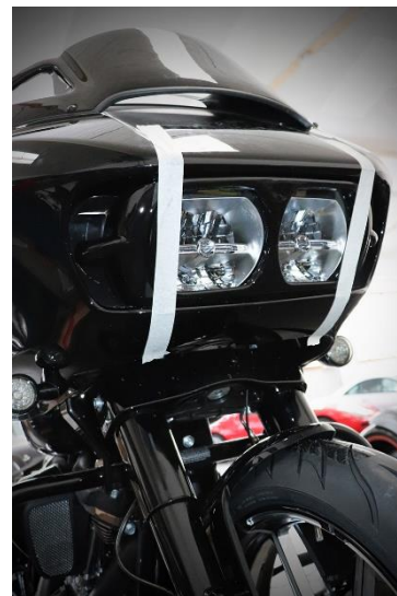
Abb. 1 & 2 – Application of mounting adhesive and temporary fastening!
