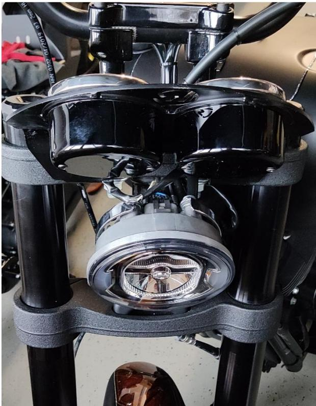
Abb. 2, Mounted speedometer set with covers
