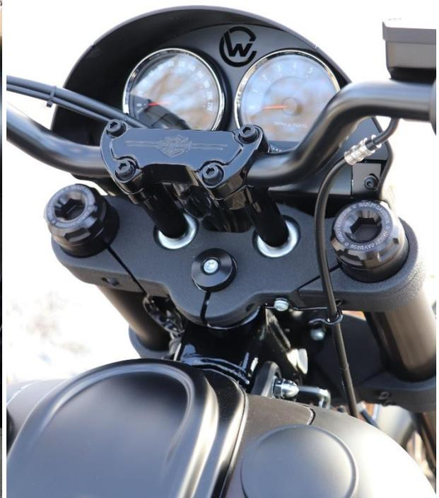
Abb. 3, Mounted speedometer set with mask
