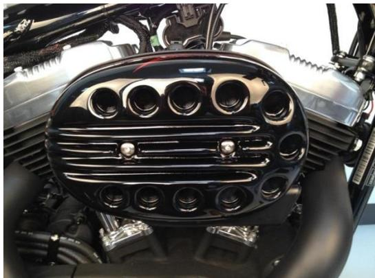
Abb. 1 – Mounted air filter cover "Slotted"
