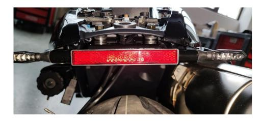
3. After that, the fastening screws (pan-head screw M6x20) can be tightened.
